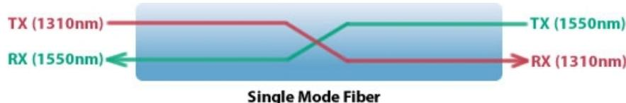
When Single Strand fiber is used, you will need an “Up” side and a “Down” side when interconnecting fiber devices.
